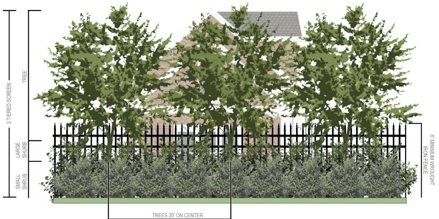
Figure 10: Alternative #2 (Wrought Iron Fence with Three (3) Tiered Screening in Perspective View)
