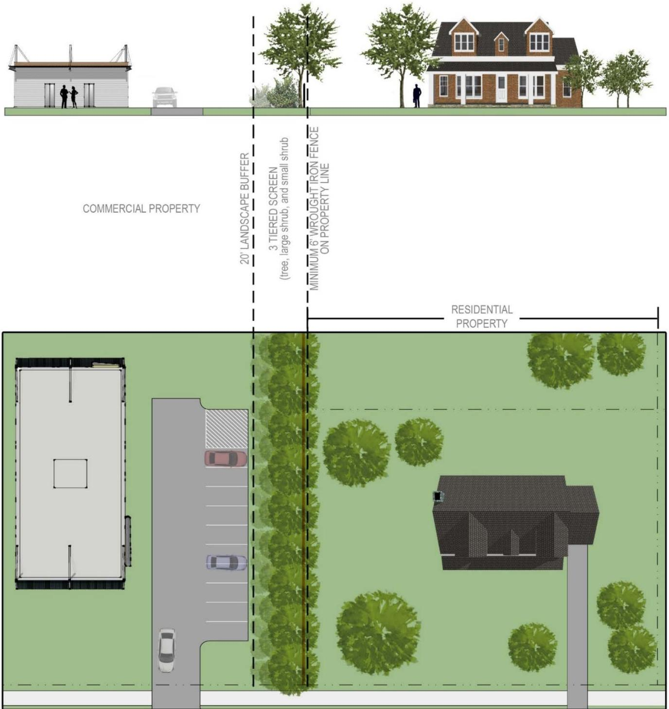
Figure 9: Alternative #1 (Wrought Iron Fence with Three (3) Tiered Screening in Perspective View)
