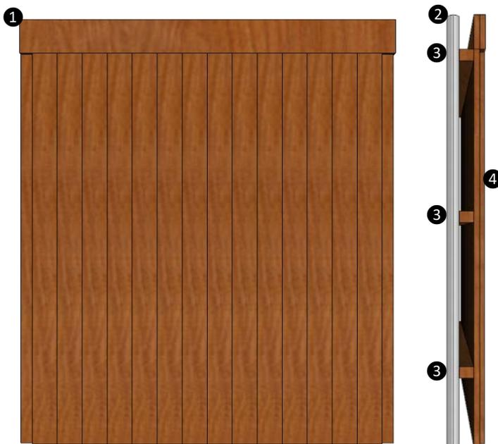
① Top Rail; ② Galvanized or Stainless-Steel Post (Recommended Minimum of  $2\frac{3}{8}$ "); ③ Stinger Board (Recommended Minimum of 2" x 3"); ④ Minimum  $\frac{1}{2}$ " Wood Screen.
