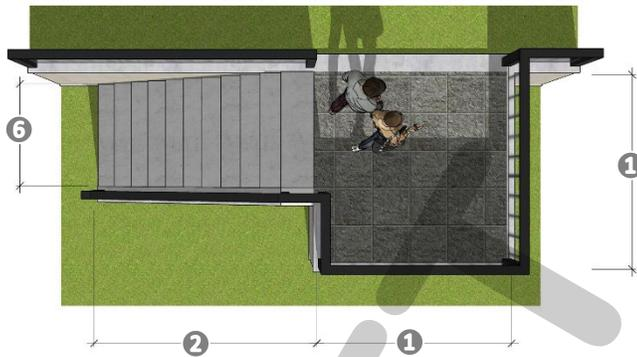
①: MINIMUM OF EIGHT (8) FOOT BY EIGHT (8) FOOT LANDING; ②: VARIABLE LENGTH STAIRCASE; ③: WROUGHT IRON OR BLACK TUBULAR STEEL; ④: NATURAL STONE, BRICK, OR CONCRETE MATCHING THE RETAINING WALL; ⑤: VARIABLE HEIGHT BUT A MINIMUM OF THREE (3) FEET; ⑥: MAXIMUM OF SIX (6) FEET.
