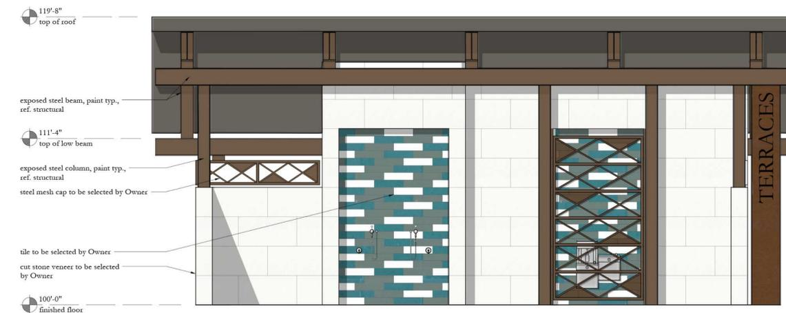
1 SOUTH ELEVATION - RESTROOM BUILDING ELEVATION
