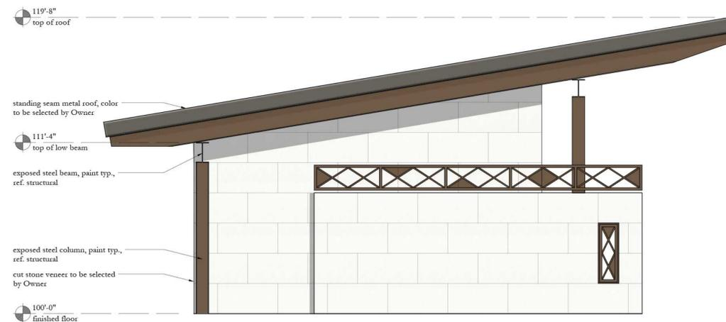
2 WEST ELEVATION - RESTROOM BUILDING ELEVATION
