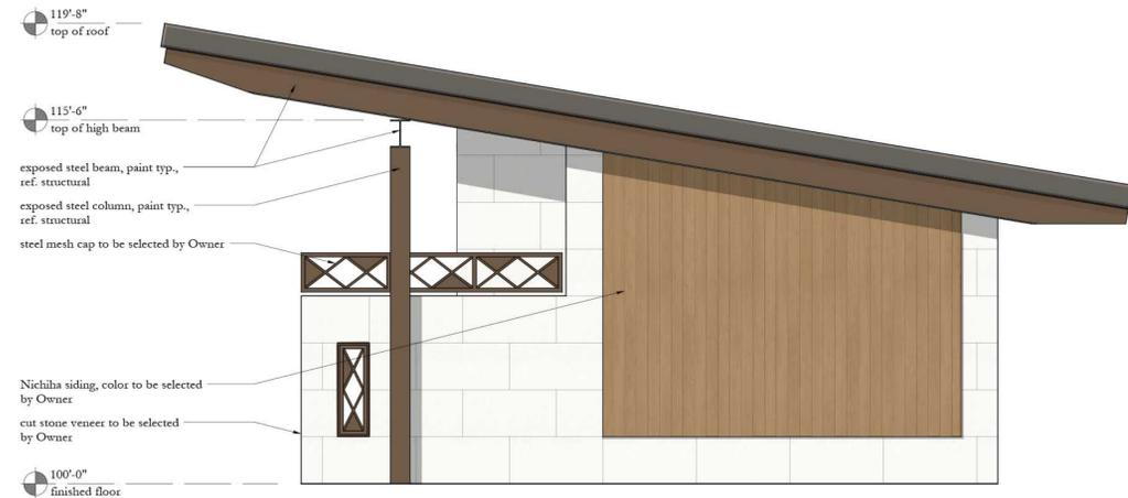
4 EAST ELEVATION - RESTROOM BUILDING ELEVATION
